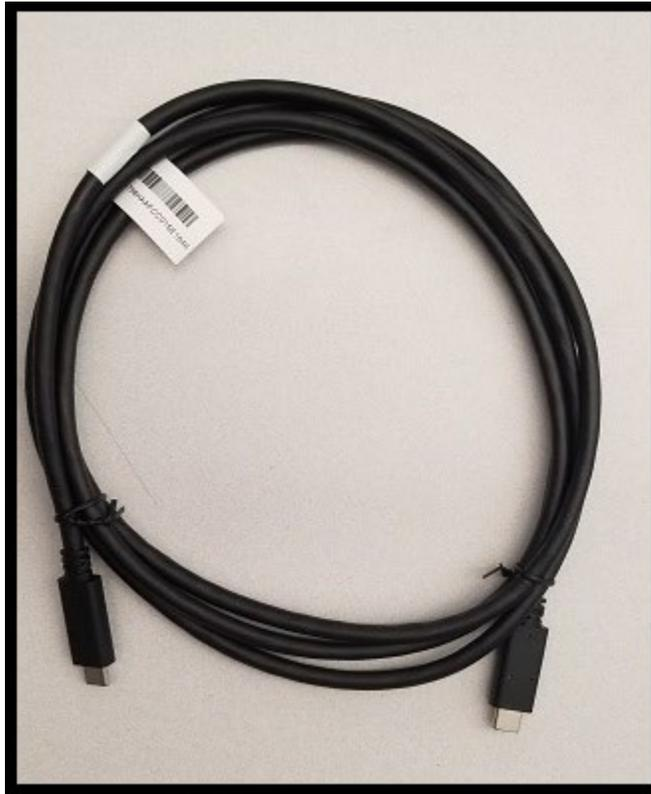
Connect one end of the **USB-C cable** to the **SS port** on the back of the **Docking Monitor**. This **SS port** is found next to the **Display Out** port on the **Docking Monitor**.
